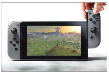
The Switch's two Joy-Con controllers attach to the sides of the device
